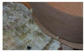
away brace wood and glue residue from the ply. I then tried to fit the back (note that I had also marked on the uke sides where the braces should be located). At first it wouldn't go, but with a very fine trim to the ends of both braces it went home with a satisfying click. After that, I carved the braces down at the ends with a sharp knife and sanded them clean.
