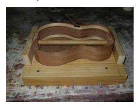
didn't have a turnbuckle lying around, but I had plenty of pieces of dowelling, so I cut a piece that just fits end to end. The picture shows the uke raised up in the mould, the razor blade caught midtrim and the dowel stretching out the uke.
