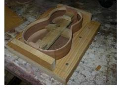
bottom down flat. This pulled the twist out of the sides. If you use this technique, make sure that the screw sits under the sound hole....mine did, the second time!
