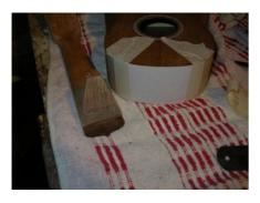
An important prep is to remove any glue residue that may have oozed out of the join between the fretboard and neck. I used a sharp blade. Then I taped sandpaper to the body and scribbled pencil on the neck gluing face of the neck, and worked the neck back and forth until most of the pencil marks had gone, indicating a flush fit.
