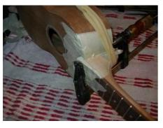
a centre sight line to get the neck alignment straight. The nut will hide the hole left when the nail is taken out.
