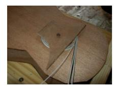
The swelling was addressed by a light sand either side to reduce the width of the glued strips. To decrease the number of fingers needed to hold the rosette, I made a spider affair (from a plywood scrap — just happened to be a good design!) and fastened it to the block under the sound hole with a screw. Tightening the screw pulls down the ply and keeps the rosette where it ought to be. In the earlier picture, the piece of ply is sitting on the uke top but has not yet been screwed into the
