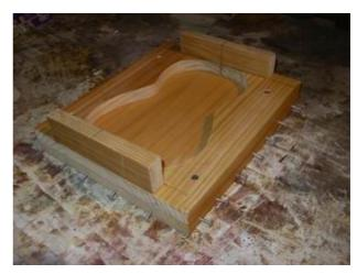
In the second picture, nails have been placed around the edge of the base. These are used to anchor the rubber bands used for clamping (the bands are supplied with the kit). Note the centreline marks on the jig.
