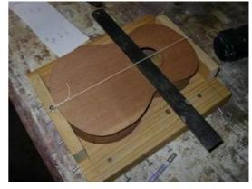
up and down on the face (not slanted). I then marked the top at the base and neck directly under the string line. From these two marks, I drew a centre line on the top.
