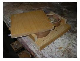
With the body completely flat I went to work with my sanding sheet. It was reasonably easy to tell when to stop – I had left the linings and sides a little proud of the neck and heel blocks, and when I could see that I was sanding the tops of the blocks I knew I was close to finished.
